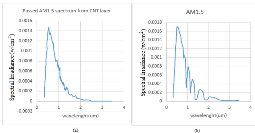
**Fig. 2.** (a) The alternative beam used in simulation, (b) The standard AM1.5 beam
