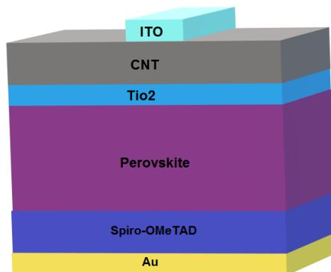
**Fig. 1.** Proposed schematic structure for perovskite solar cell.
