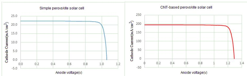
**Fig. 3.** I-V characteristics for simple and CNT based perovskite solar cell.
