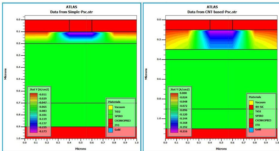
**Fig. 4.** Total current density in simple perovskite solar cell and CNT based perovskite solar cell.
