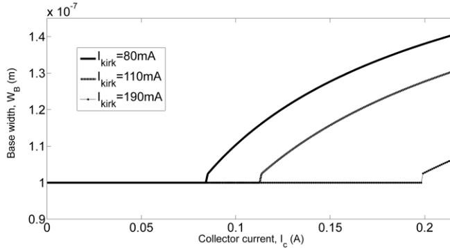
**Fig. 2.** Modified base width versus collector current, for different kirk current.
