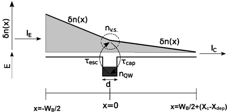
**Fig. 1.** Schematic of carrier diffusion and quantum capture in the quantum wells, and the conduction band energy of the base region.
