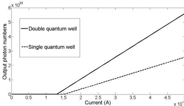
**Fig.7** Output photon numbers versus base current for transistor laser with single and double well
