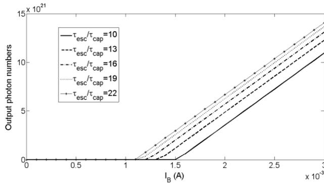
**Fig.6** Light-current characteristics versus base current for different quantum capture efficiency
