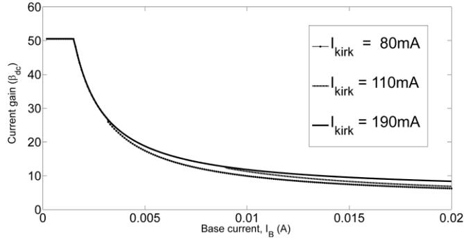
**Fig. 3.** DC current gain versus base current for different kirk current.
