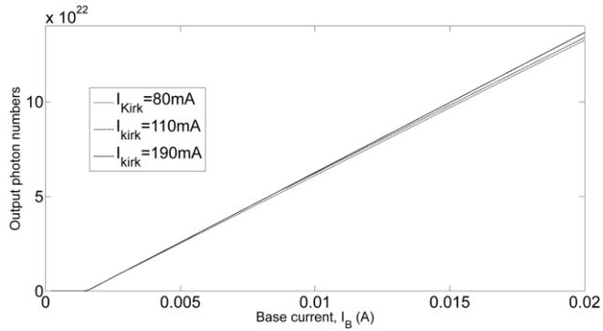
**Fig.4** Light-current characteristics versus base current for different kirk current.
