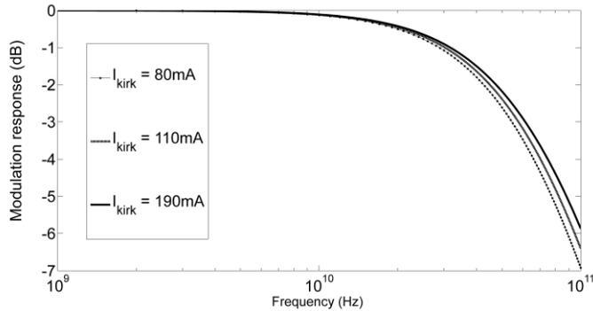
**Fig.8** Modulation response versus frequency for transistor laser with different kirk currents.
