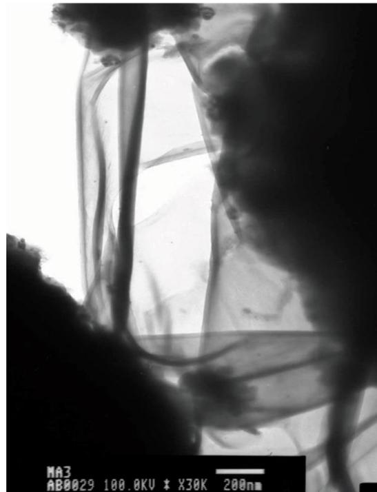
Fig. 6. SEM image of the graphene layers over MCM-41 catalyst.
