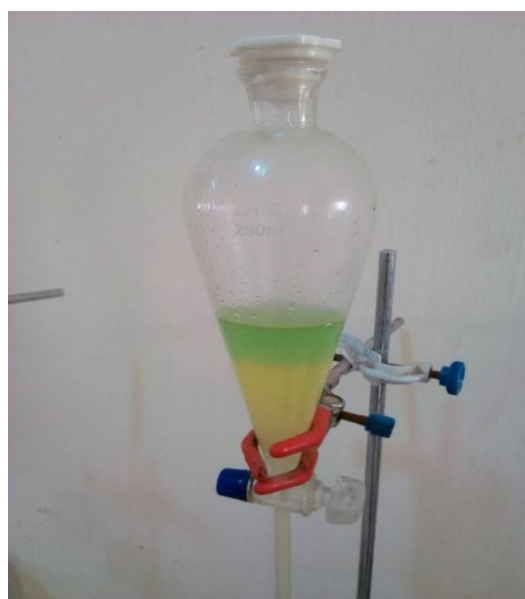
Figure 2. The collected sample showing the biodiesel layer on top and glycerol at the bottom
