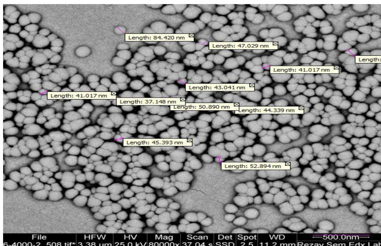
Fig.6. SEM image of silver nanoparticles synthesized from Peel Oak extract
