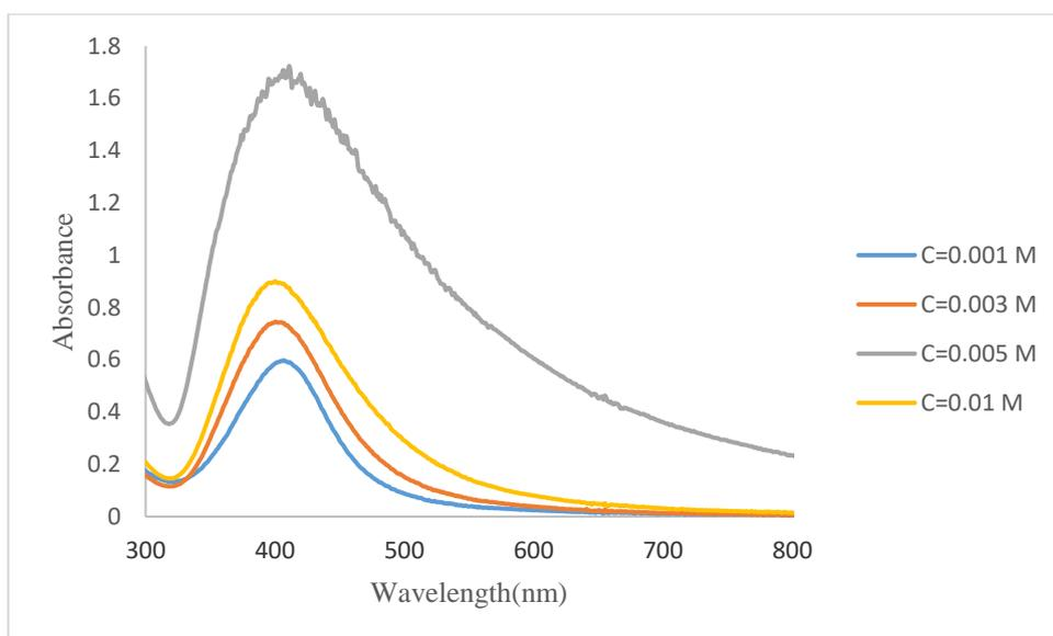
Fig.3. Effect of silver nitrate concentration on silver nanoparticles synthesis by Peel Oak extract (2ml extract solution, pH=8, stirring rate 150rpm, time: 30 min)
