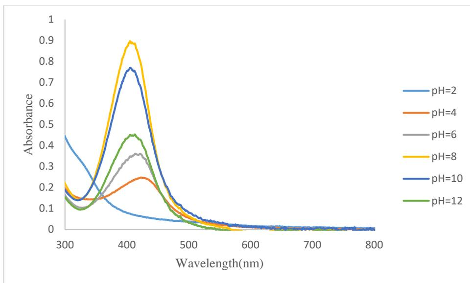
Fig.2. Effect of pH on silver nanoparticles synthesis by Peel Oak extract (32ml Agno<sub>3</sub> 0.001M, 2ml extract solution, stirring rate 150rpm, time: 30 min)
