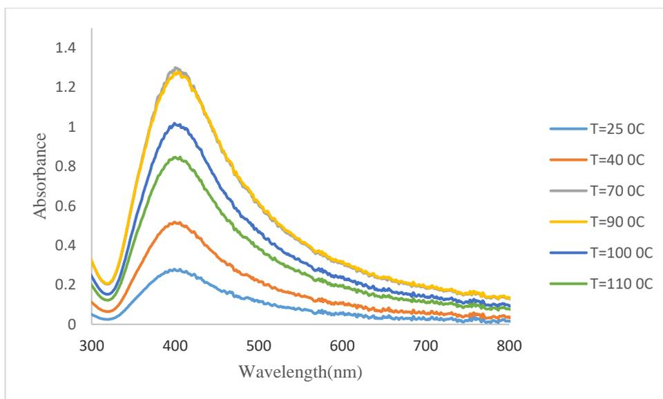
Fig.4. Effect of temperature on silver nanoparticles synthesis by Peel Oak extract ( 2ml extract solution, 32 ml silver nitrate concentration 0.005M, pH=8, time:30 min)
