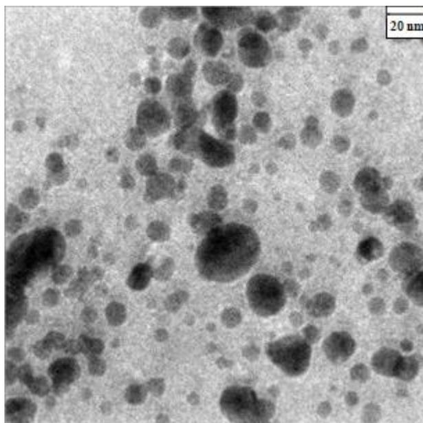
Fig. 7. TEM image of synthesized silver NPs using *Peel Oak* extract
