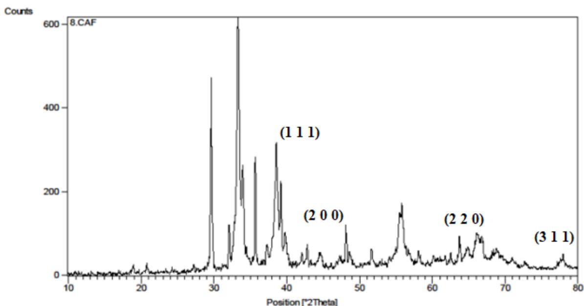
Fig. 8. XRD pattern of synthesized silver NPs using *Peel Oak* extract
