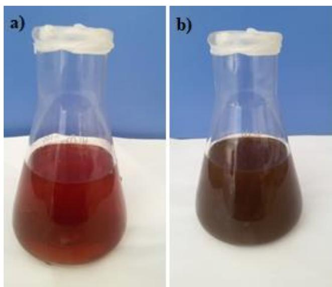
Fig 1. a) Peel Oak pure extract; b) Colloidal solution of silver nanoparticles after reduction of silver nitrate by Peel Oak extract
