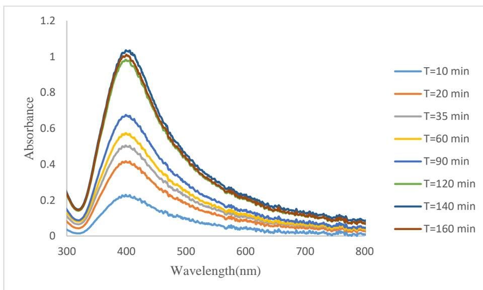
Fig.5. Effect of contact time on silver nanoparticles synthesis by Peel Oak extract ( 2ml extract solution, 32 ml silver nitrate concentration 0.005M, pH=8, temperature:90 °C)
