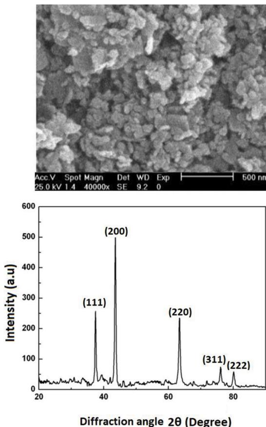
Fig. 1. The SEM picture (up) and the XRD pattern (down) of synthesized CaO nanoparticles.
