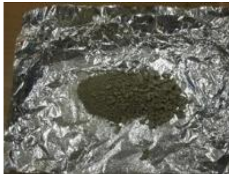
Fig 2 Grinding lumped silicon carbide on aluminum foil.
