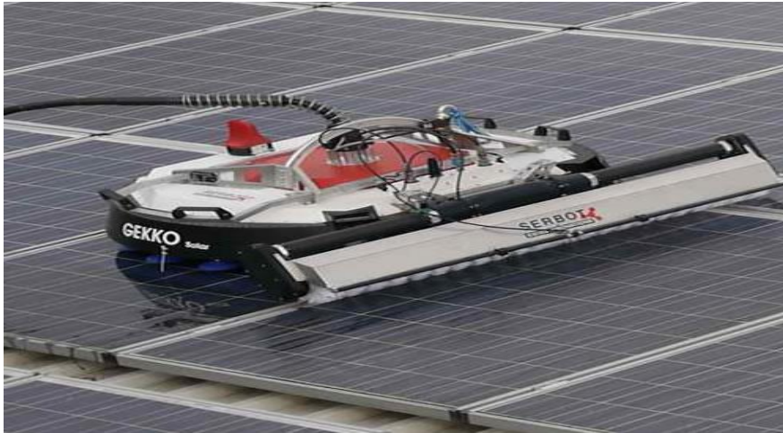
Fig. 9 . Cleaning using Gekko solar and Gekko solar farm [17]
