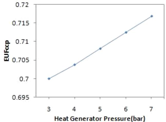
Fig. 12. Effects of generator pressure variations on EUF<sub>ccp</sub>.
