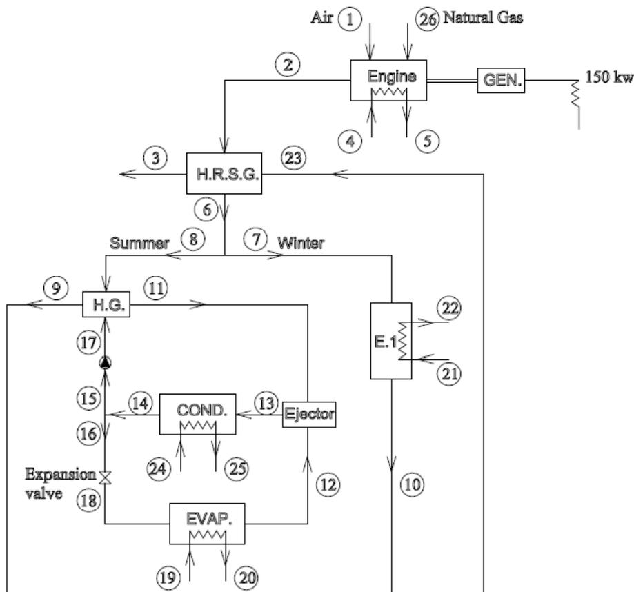
**Fig. 1. Simplified schematic view of a simultaneous power, cooling and heating energy generating system driven by an internal combustion engine and a steam ejector refrigeration system.**
