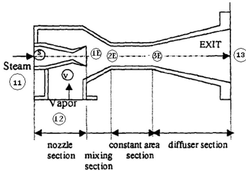
Fig. 3. Schematic view of an ejector.
