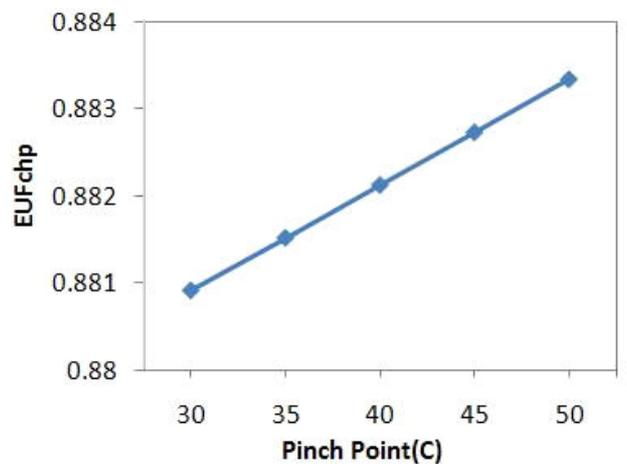
Fig. 5. Effects of pinch point temperature variations on EUF<sub>chp</sub> for winter.
