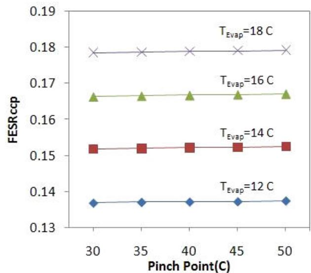
Fig. 8. Effects of pinch point temperature on FESR<sub>ccp</sub> for different evaporator temperatures for winter.
