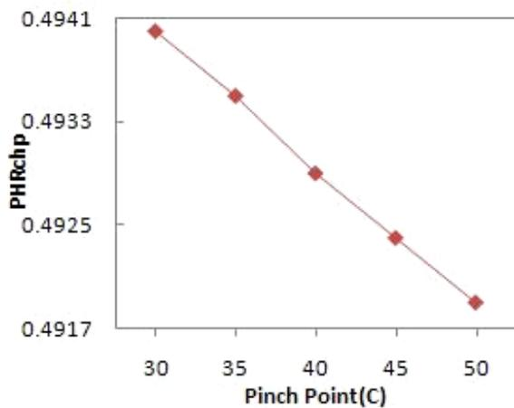
Fig. 10. Effects of pinch point temperature variations on PHR<sub>chp</sub> for winter.
