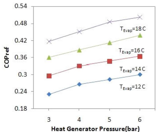
Fig. 9. Effects of generator pressure variations on COP<sub>pref</sub> for different evaporator temperatures.
