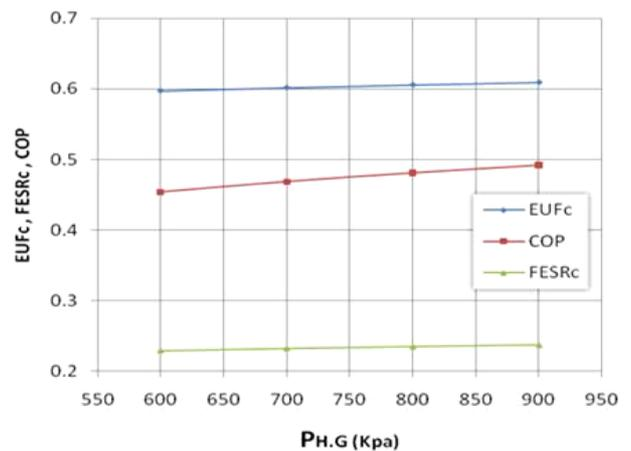
Fig. 13. Effects of heat generator pressure of ejector on total efficiency of cycle, fuel energy saving ratio (in generating power and cooling modes), and coefficient of steam ejector refrigeration system performance [15].
