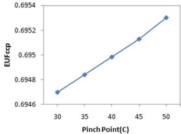
Fig. 4. Effects of pinch point temperature variations on EUF<sub>ccp</sub> for summer.
