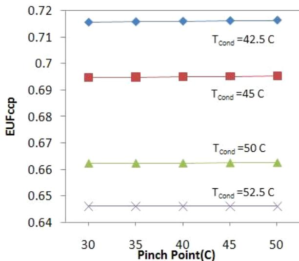
Fig. 6. Effects of pinch point temperature on EUF<sub>ccp</sub> for different condenser temperatures for summer.
