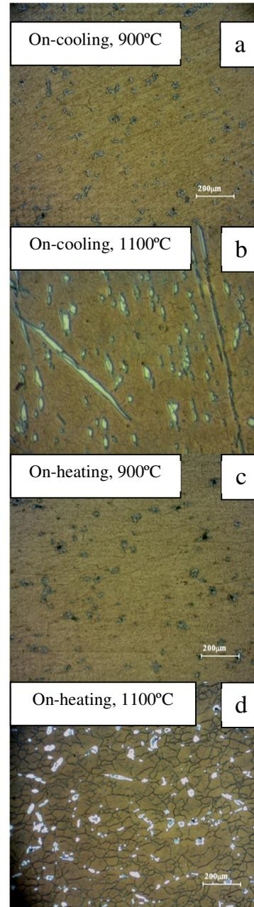
**Fig.6.** Microstructures of hot deformed steel C1 at 900°C and 1100°C. The dark phase is ferrite and the light one is austenite
