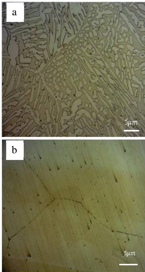
**Fig.2.** Microstructure of homogenized samples (a) C2 (The light phase is austenite and the matrix is ferrite) (b) C1 (Essentially ferritic microstructure).
