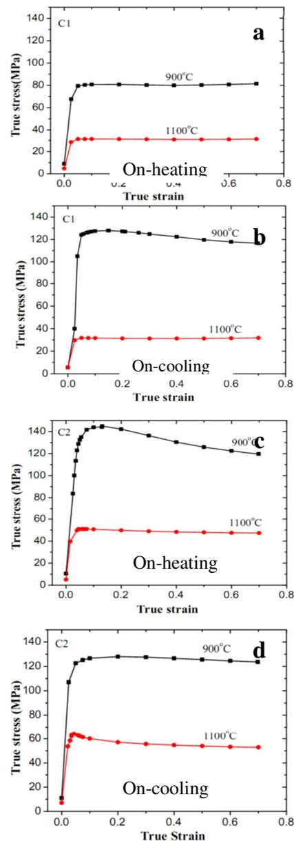
**Fig.4.** True stress-strain curves for steels C1 and C2 under different deformation condition with strain rate of 0.1 sec<sup>-1</sup>.
