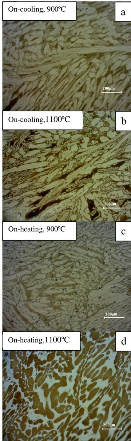
**Fig.7.** Microstructures of hot deformed steel C2 at 900 °C and 1100°C. The dark phase is ferrite and the light one is austenite.
