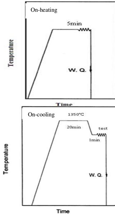
**Fig.1.** Schematic of heat treatment cycles.
