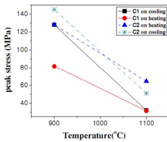
**Fig.5.** Dependence of the peak stress on deformation temperature for steels C1 and C2.
