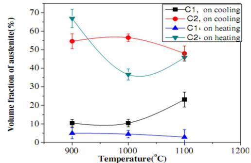
**Fig.3.** Dependence of austenite volume fraction on deformation temperature for cycles 1 and 2.
