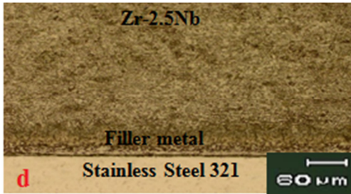
Fig. 3. Optical microscopy image of brazed joint: (a) 850°C, 10min (b) 850°C, 15 min (c) 865°C, 10min,(d) 865°C, 15min.
