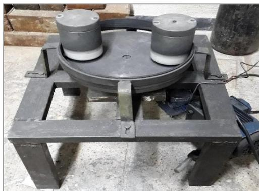
**Fig. 1.** The high-energy planetary ball mill.
