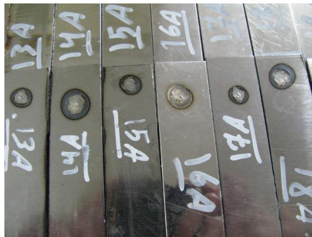
Fig.1. Resistance spot welded specimens according to table 4 experiments.
