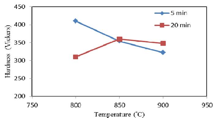
**Fig. 12.** Hardness of the samples annealed for 5 and 20 min at 800, 850, and 900 °C after rolling
