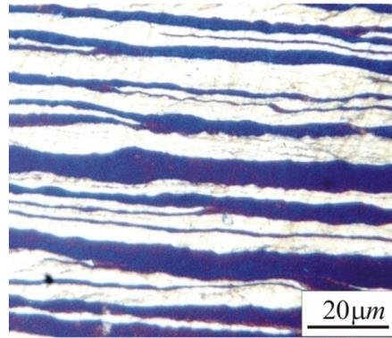
**Fig. 3.** Microstructure of the rolled DSS (TD direction)
