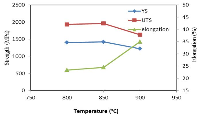
**Fig. 11.** Ultimate tensile strength (UTS) and yield strength (YS) and elongation of the samples annealed for 20 min at 800,850 and 900 °C
