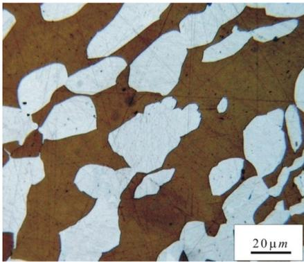
**Fig. 2.** Microstructure of the as-cast DSS after solution treatment at 1200 °C for 60 min and water quenching
