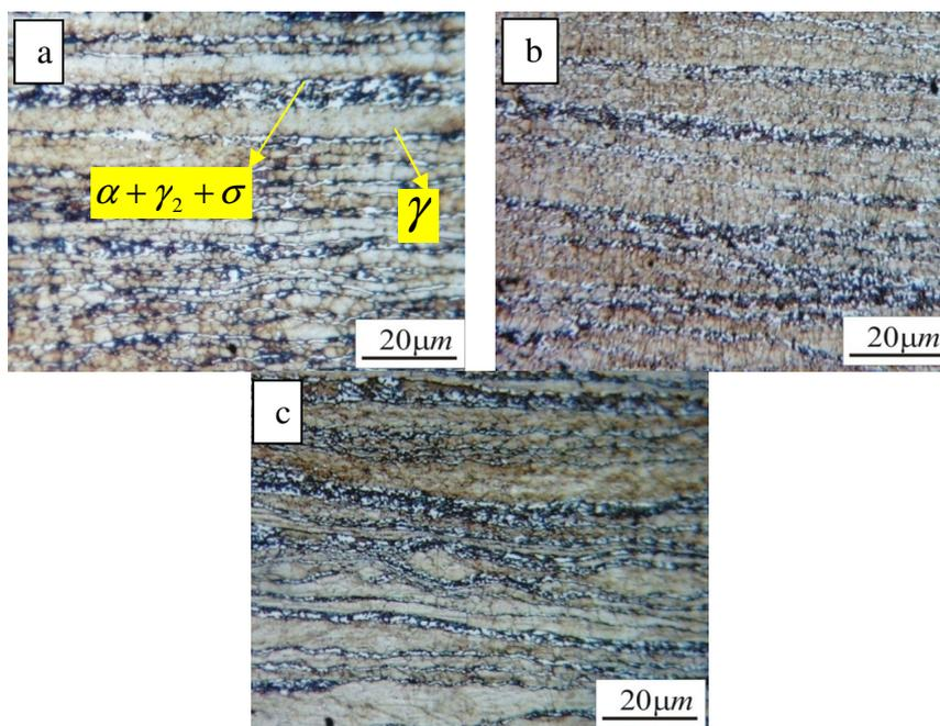
**Fig. 6.** Microstructure of cold rolled DSS with annealing at temperature a) 800, b) 850, and c) 900 °C for 20 min
