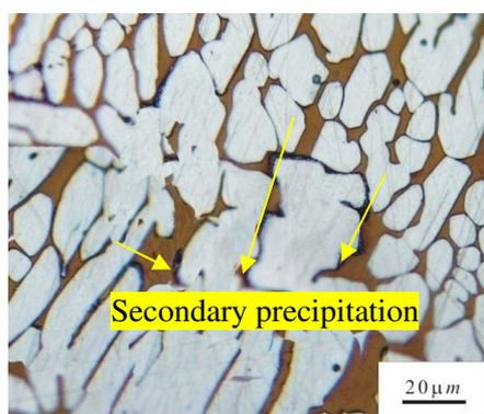
**Fig. 1.** Microstructure of the as-cast DSS
