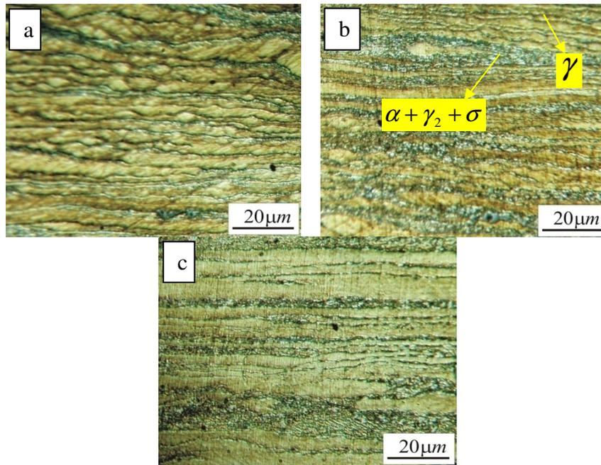
**Fig. 5.** Microstructure of the cold rolled DSS with annealing at temperature a) 800, b) 850, and c) 900 °C for 5 min
