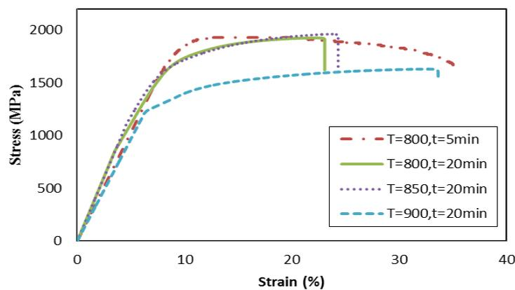
Fig. 10. Engineering stress-strain curve of the cold rolled and annealed samples
