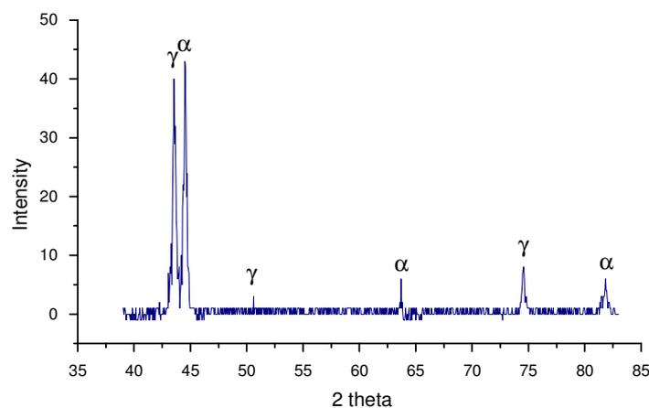
**Fig. 4.** X-ray diffraction of the cold rolled specimen
