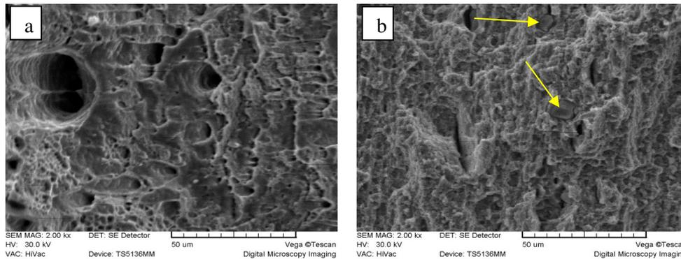
**Fig. 13.** Fracture surfaces of rolled samples: a) without anneal, b) annealed for 20 min at 800 °C
