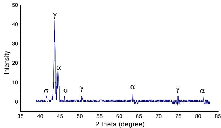
Fig. 8. X-ray diffraction of sample annealed at  $800^{\circ}\text{C}$  for 5 min
