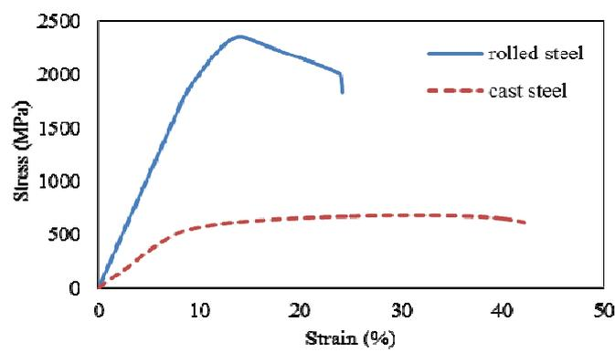
Fig. 9. Engineering stress-strain curve of the cold rolled sample (without annealing) and the cast steel
