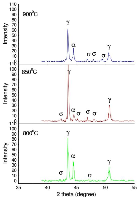
**Fig. 7.** X-ray diffraction of the samples annealed at 800,850 and 900 °C for 20 min
