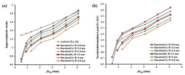
**Fig. 4.** The effect of  $\Delta r_{die}$  and R on: (a) Imposed plastic strain and (b) needed deformation load through TCP processing
