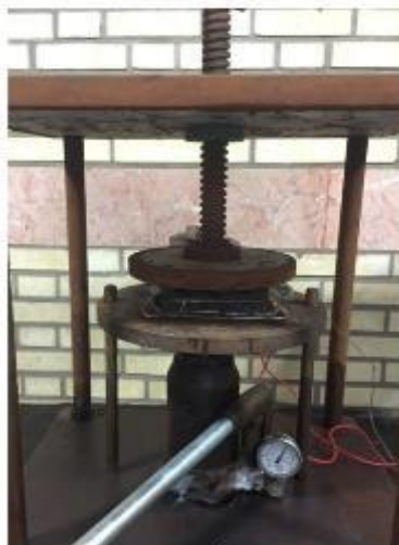
Fig. 4. Hot-press machine used for composite fabrication
