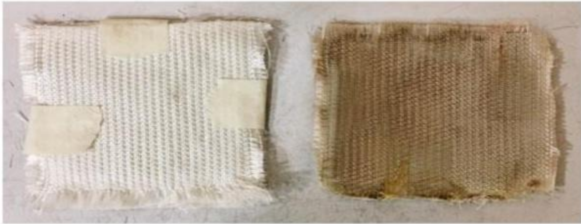
Fig. 5. Composite laminate before and after the hot-pressing process
