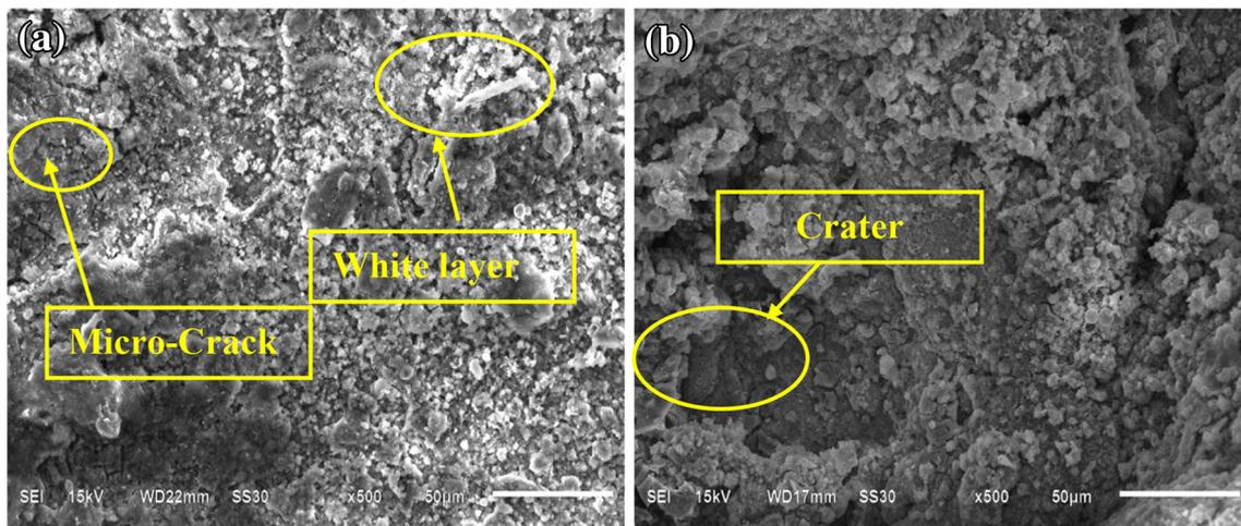
**Fig. 10** a, b SEM micrograph of drilled surface
