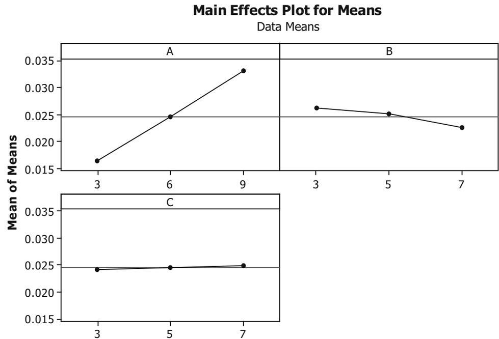
**Fig. 5** Main effects plot for means (TWR)
