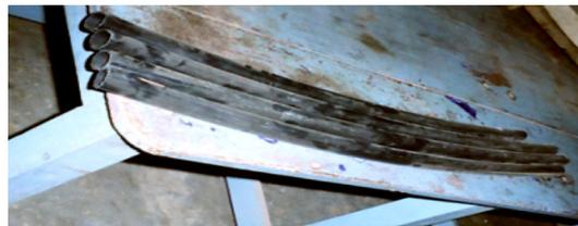
Fig. 3 The extruded HDPE pipes
