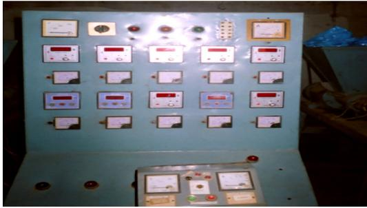
**Fig. 5** Panel board showing different zone temperatures
