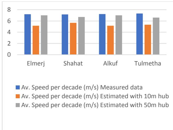
Fig. 6. Average measured, estimated at 10m, and 50m wind speed.
