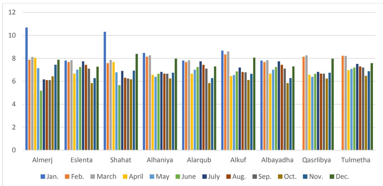
Fig .5. The Monthly Measured Wind Speed (m/s) Averaged over a Decade at 9 Sites
