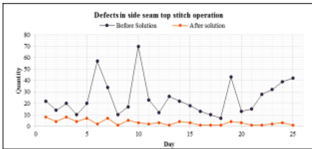
Fig. 13. Defect level before and after corrective actions for side seam top stitch operation
