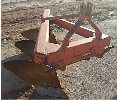
Fig. 1. The three-bottom mounted moldboard plow used in this study.
