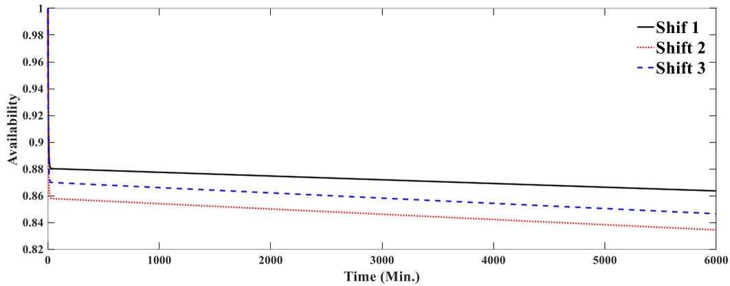
Fig. 3. Availability diagram of different shifts with repairable subsystems
