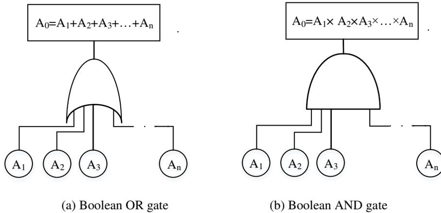
Fig. 2. Fault tree representation
