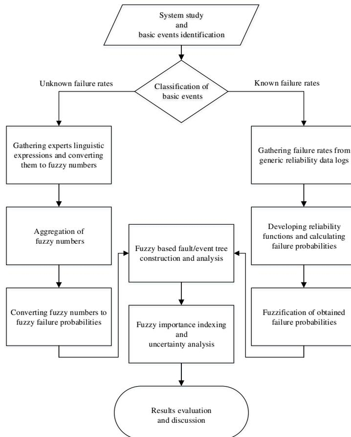
Fig. 1. Chart of fuzzy based PSA for HWRR
