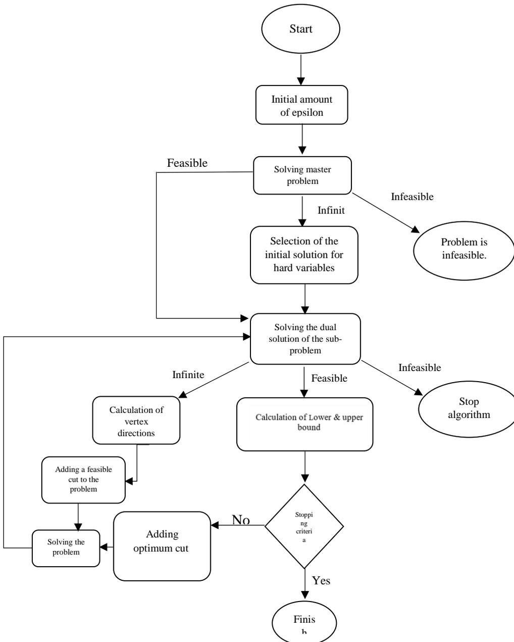
Fig. 1. Benders' decomposition algorithm
