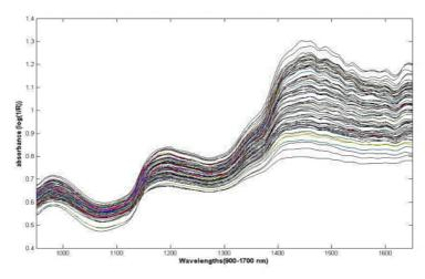
Fig. 1. Raw NIR spectra of sugar beet samples
