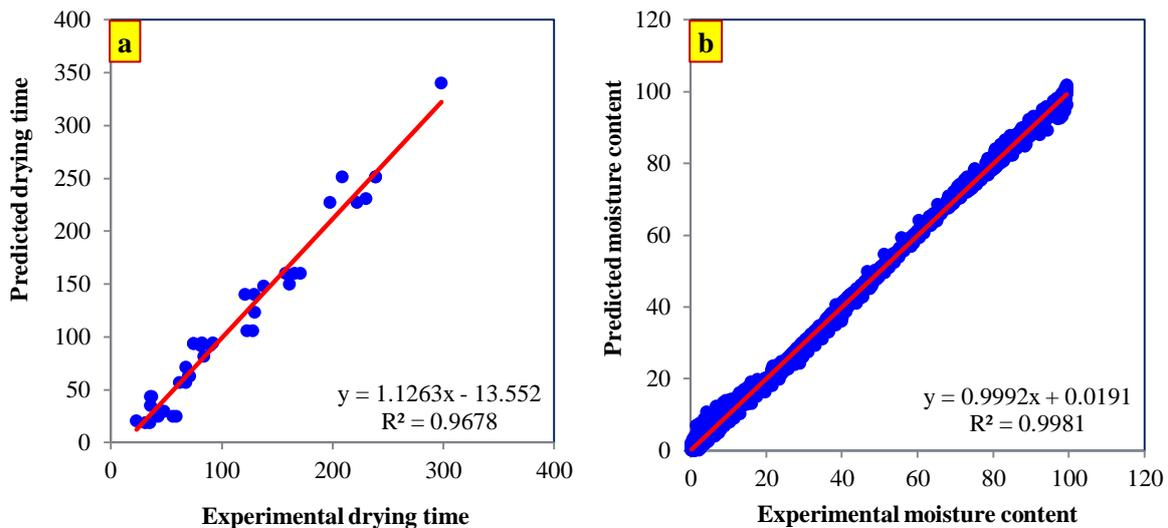
**Fig. 1.** Experimental versus predicted values of drying time (a) and moisture content (b) using GA-ANN model
