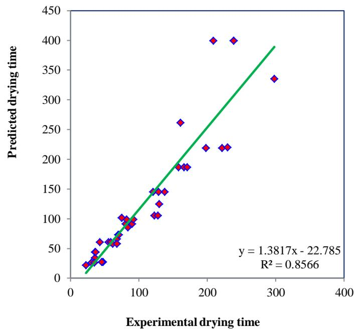
**Fig. 5.** Experimental versus predicted values of drying time using the ANFIS model.
