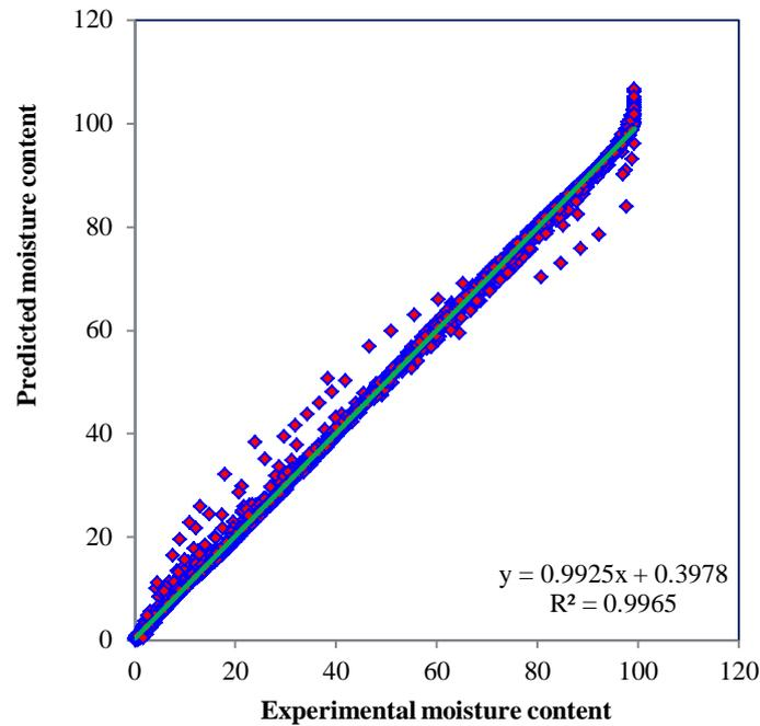
**Fig. 6.** Experimental versus predicted values of moisture content using the ANFIS model
