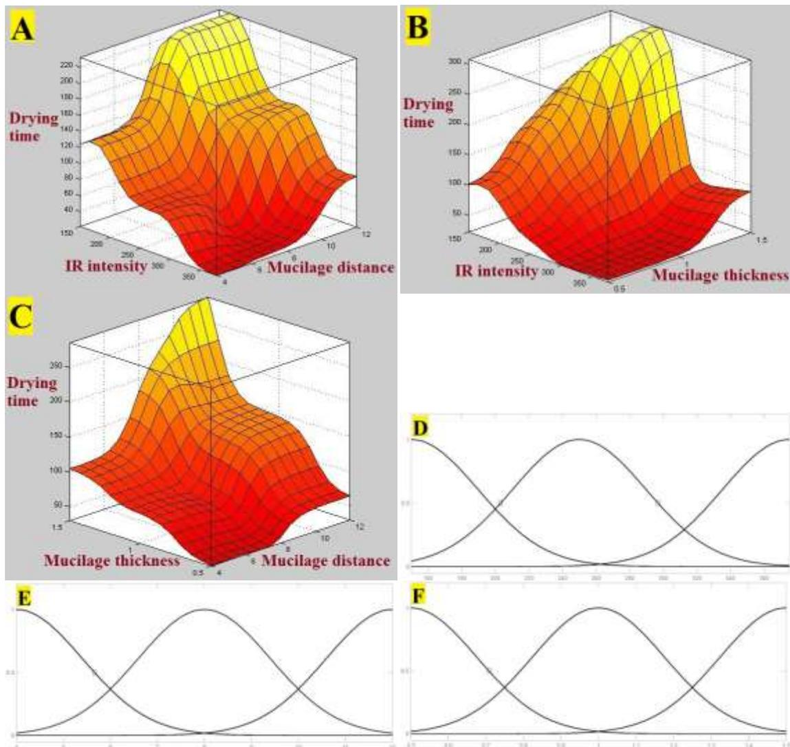
**Fig. 4.** Response surface diagram for (a) IR power & mucilage distance, (b) IR power & mucilage thickness and (c) mucilage distance & mucilage thickness versus drying time. (D), (E) and (F) the membership functions of IR power, mucilage distance and mucilage thickness, respectively.
