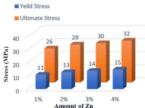
Fig. 6. The compressive strength of the synthesized scaffolds containing of different Zn amounts.
