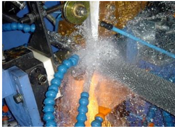
Fig. 13. The welding process currents of high frequency [13].
