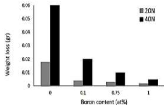
Fig. 3. the variation of weight loss of the samples after 1000 m of dry sliding test.
