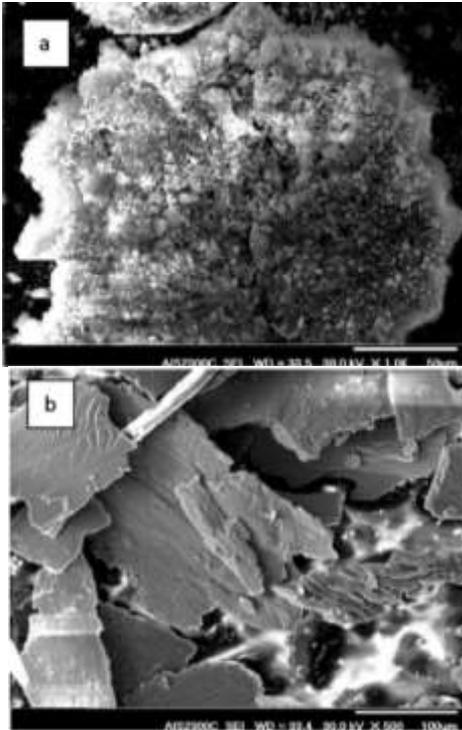
**Fig. 7.** SEM image of the a) oxide particles and b) fresh metallic particles removed from the surface during the wear.
