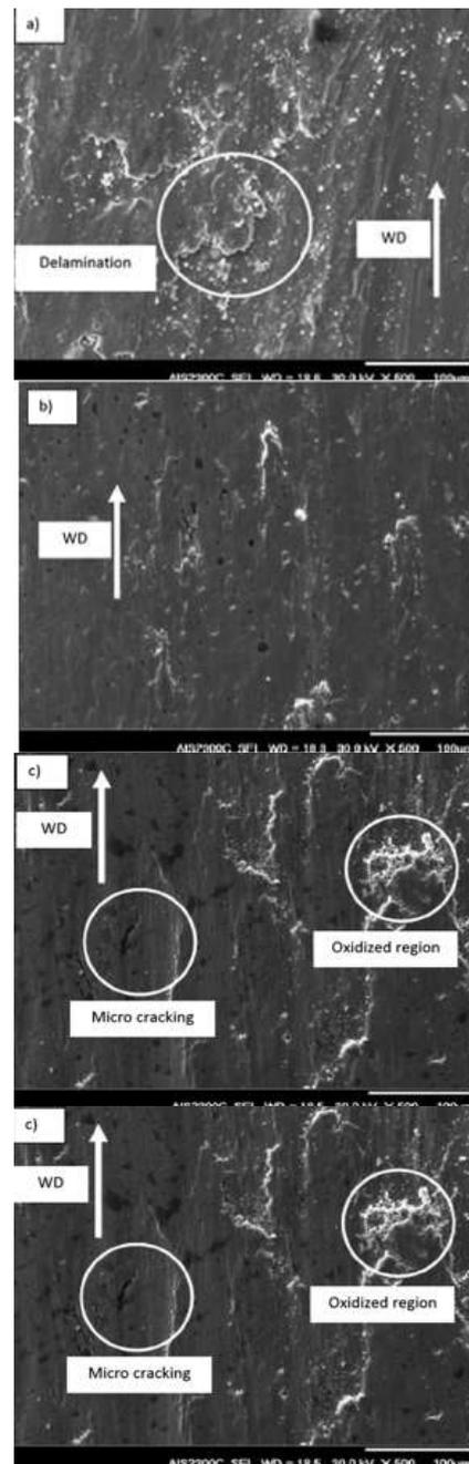
Fig. 6. The worn surface of the materials at the load of 40 N a) FeAl b) FeAl-0.1B, c) FeAl-0.75B d) FeAl-1B.
