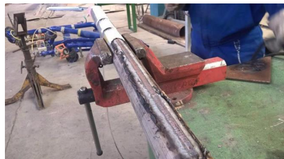
Fig. 2. Welded pipe before cleaning.
