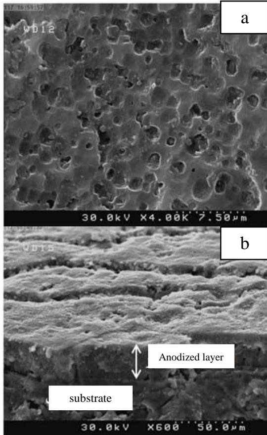
**Fig. 1. FESEM images of a) surface morphology and b) cross-section of single-layer anodizing coating.**
