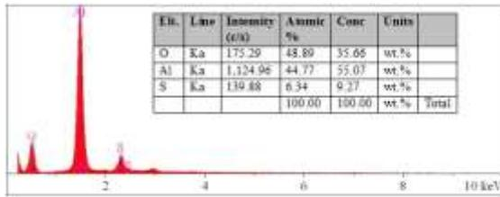
Fig. 4. The results of EDS analysis of the single-layer anodized coating surface.
