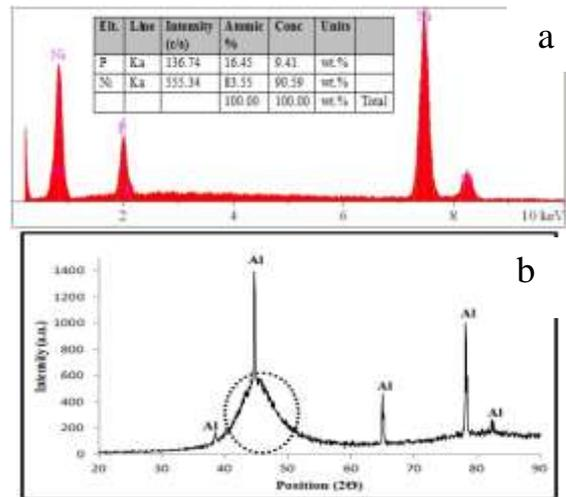
Fig. 6. The results of a) EDS analysis and b) X-ray diffraction pattern of anodized/nickel-phosphorus hybrid coating without heat treatment.
