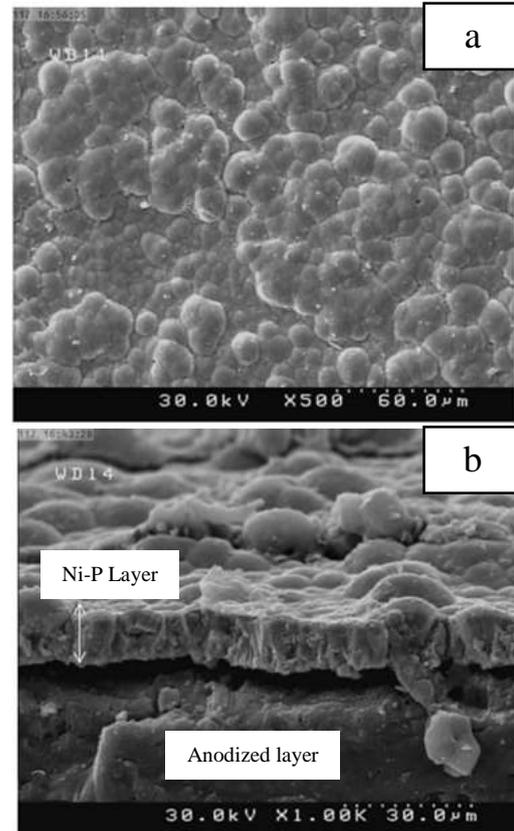
**Fig. 3. FESEM images of a) surface morphology b) cross section of electroless nickel-phosphorus coating.**
