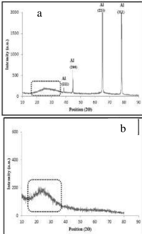
Fig. 5. Diffraction pattern results obtained from a) XRD test and b) GIXRD test of single-layer anodized coating.
