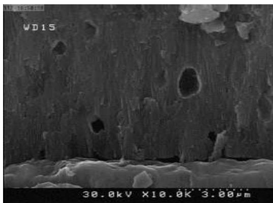
**Fig. 2. FESEM image of the cross section of the anodized layer including the grown Nanocells.**
