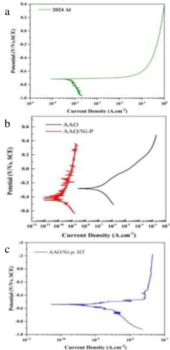
**Fig. 8. The obtained potentiodynamic polarization diagram related to a) aluminum 2024 b) single-layer and hybrid coatings c) heat-treated hybrid coatings after 2 hours of immersion in 3.5 wt.% NaCl solution.**
