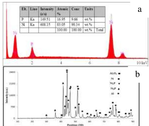
Fig. 7. The results of a) EDS analysis and b) XRD tests of anodized/nickel-phosphorus hybrid coating after heat treatment.
