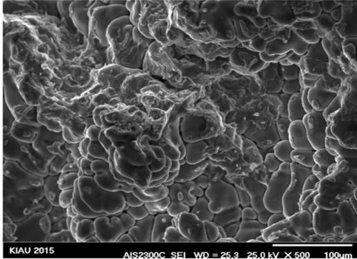
**Fig. 3.** SEM image of A201 teared surface casted in CO<sub>2</sub> sand mold.
