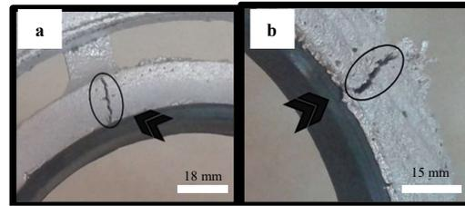
**Fig. 2. Formation of hot tears in a) ring No. 2 of CO<sub>2</sub> sand mold, b) ring No. 3 of green sand mold.**
