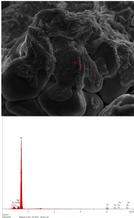
**Fig. 4.** EDAX analysis of A201 alloy sample.
