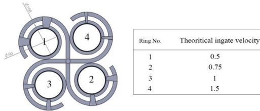
**Fig. 1. Ring mold design for hot tearing susceptibility evaluation.**
