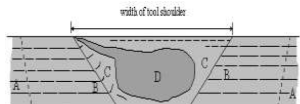
Fig. 5. The system divides the weld zone into distinct regions: A. Unaffected material B. Heat affected zone (HAZ) C. Thermo-mechanically affected zone (TMAZ) D. Weld nugget (Part of thermo-mechanically affected zone).
