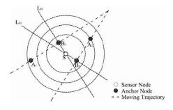
Fig. 2. Determination of sensor node location
