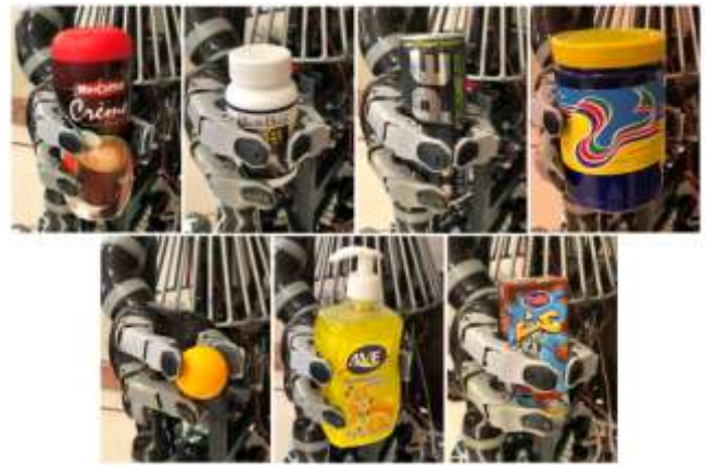
Fig. 13. Grasping object with differences in geometry and mass by the robotic arm.
