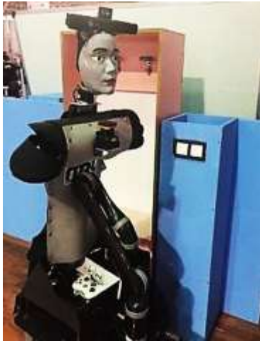
Fig. 2. The JACO mounted on the mobile autonomous robot as an assistive robotic arm, in at home MRL laboratory.
