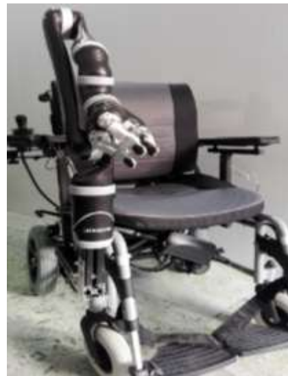
Fig. 1. The six degrees of freedom of JACO mounted on the wheelchair as a assistive robotic arm, [14].
