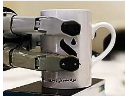
Fig. 3. Grasping of the object by JACO and its 3-finger hand
