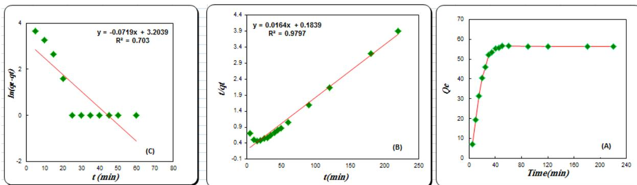
Figure 8. The effects of reaction time (A), first-order (B) and, second-order on Congo red (CR) dye.
