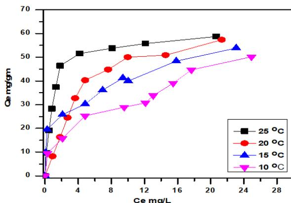
**Figure 6.** Adsorption isotherms of Congo red (CR) dye on PLAC at several temperatures.
