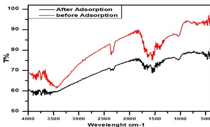
Figure 2. FT-IR spectra of PLAC before and after adsorption of Congo red (CR) dye.
