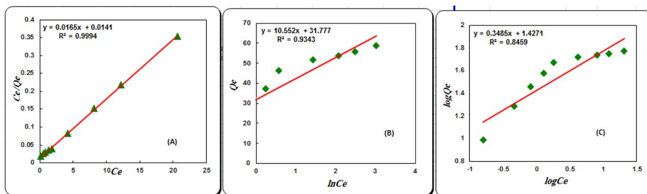
**Figure 7.** Isotherm Langmuir (A), Isotherm Freundlich (B), and Isotherm Temkin (C) of CR dye adsorption on AC.
