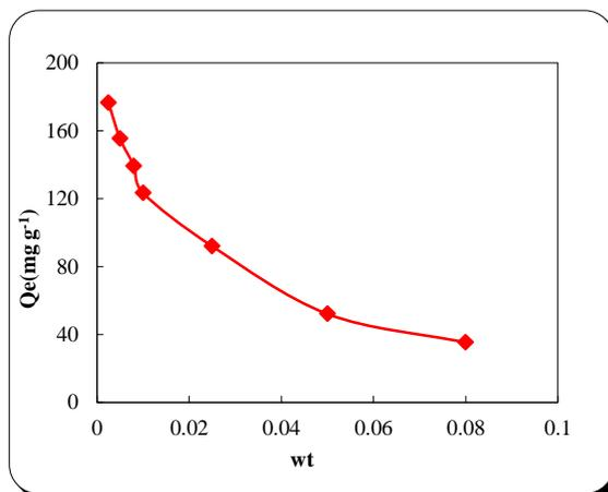
**Figure 4.** Effects of the weight adsorbent (PLAC) on the amount of adsorbed CR dye (primary concentration of the dye = 30 mg L<sup>-1</sup>, contact time 1 hr and T = 20°C)
