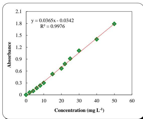
Figure 1. Calibration curve of Congo red (CR) dye.
