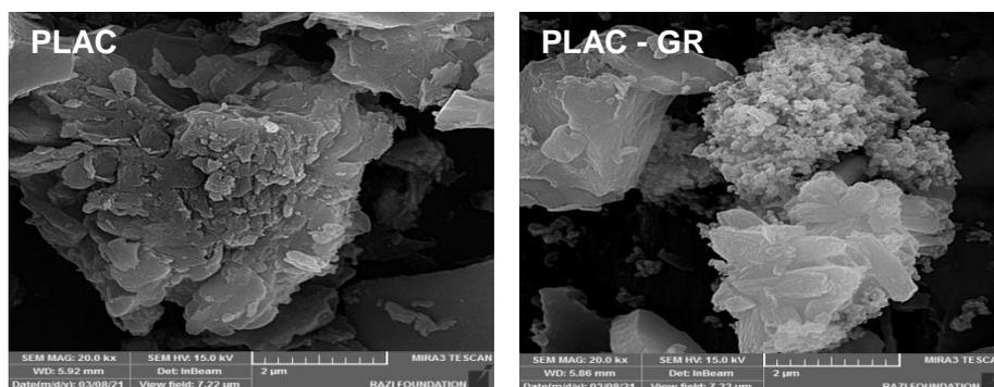
Figure 3. FESEM image of AC before and after and the GR dye adsorption.
