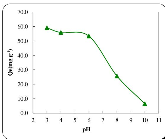
**Figure 5.** Effects of solution pH on the CR dye adsorption on AC. (optimum Condition: concentration = 30 mg L<sup>-1</sup>, a mass of AC 0.05 gm and T. = 20°C).
