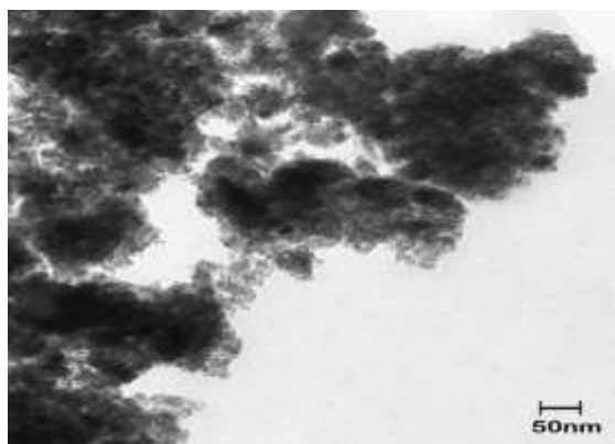
Figure 2. TEM images of Fe 3 O 4 nanoparticles before coating with dithiooxamid.
