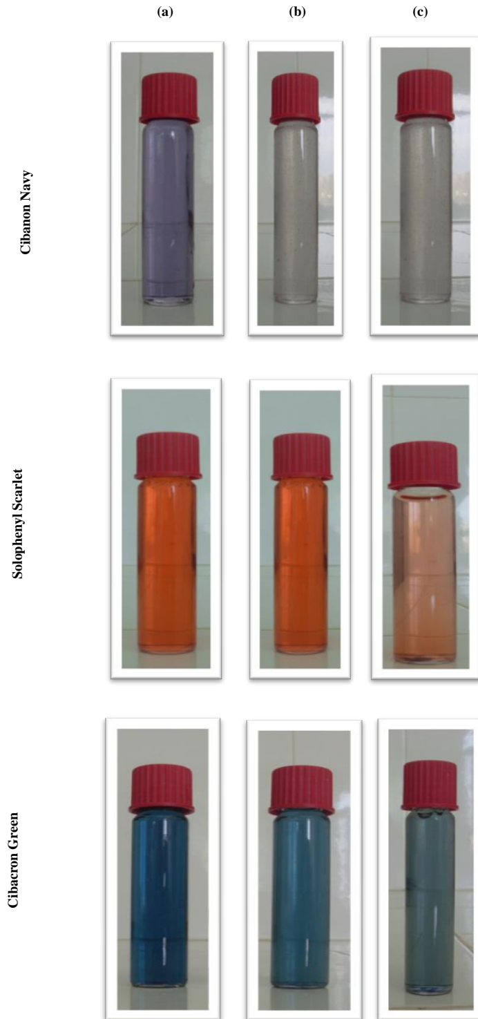
Figure 3. Discolorisation of dye solution by the activated sludge. (a) Before treatment, (b) After treatment without glucose, (c) After treatment with glucose
