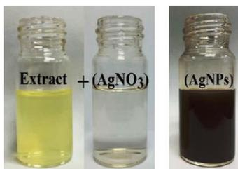
Figure 1. A: plant extract B: AgNO<sub>3</sub> solution, C: Silver Nano Particle.
