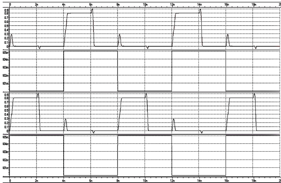
Figure 6. Waveforms of proposed comparator
