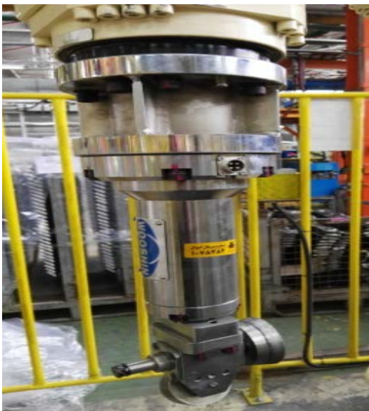
Fig.10. Robot's roller hamming section
