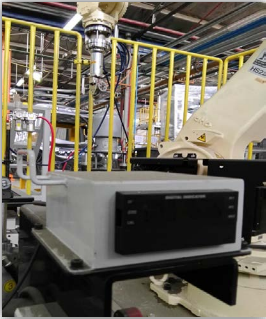
Fig.11. Load Cell section to adjust robot pressure
