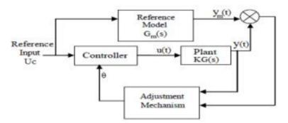
Fig.1. Model Reference Adaptive Control System
