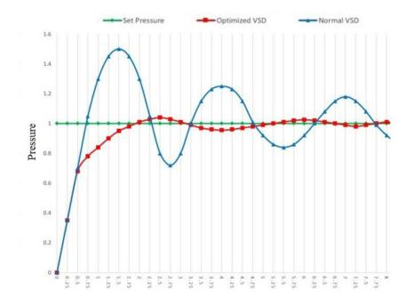
Fig.6. Comparison of output pressure of VSD and optimized VSD
