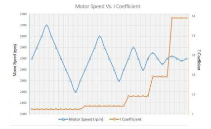
Fig.3. Effects of variation of "I" coefficient magnitude on motor speed vibrations
