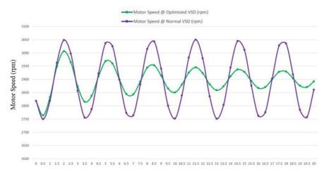
Fig.7.Comparison of speed of VSD and optimized VSD electro-motor
