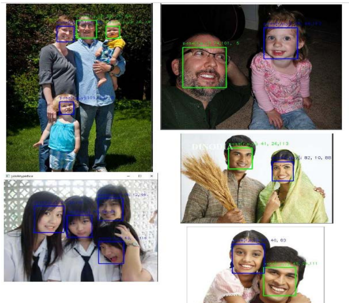
Figure 10. Qualitative results of the proposed method (The blue boxes represent the recognized faces of the women and the pink boxes represent the recognized faces of the man. Pose estimation on each face is shown at the top of these boxes for rotation, up and down bending, and left and right bending, respectively)
