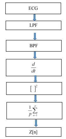
Fig.3. The Algorithm of pantompekins
