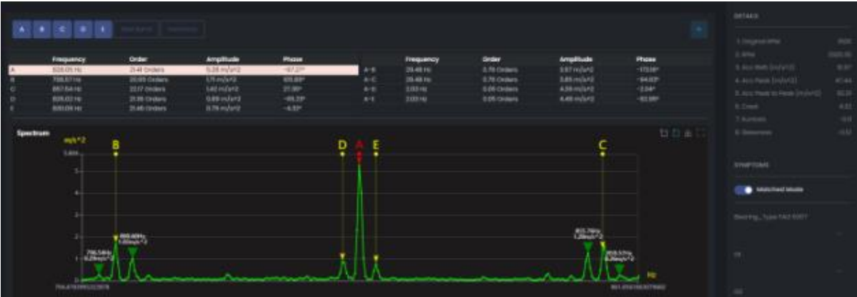
Fig.3. Magnified Horizontal -Acceleration Spectrum including lay-shaft speed and hunting tooth frequencies sidebands around 2 nd harmonic of Gear Mesh Frequency
