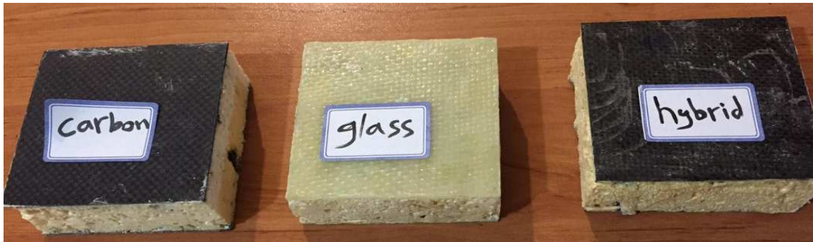
Fig.9. [C]_s , [G]_s , and [CGCG]_s composite sandwich panels with polyurethane foam
