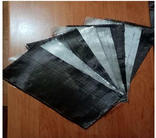
Fig.1. [CGCG]s arrangement for FRP hybrid composite
