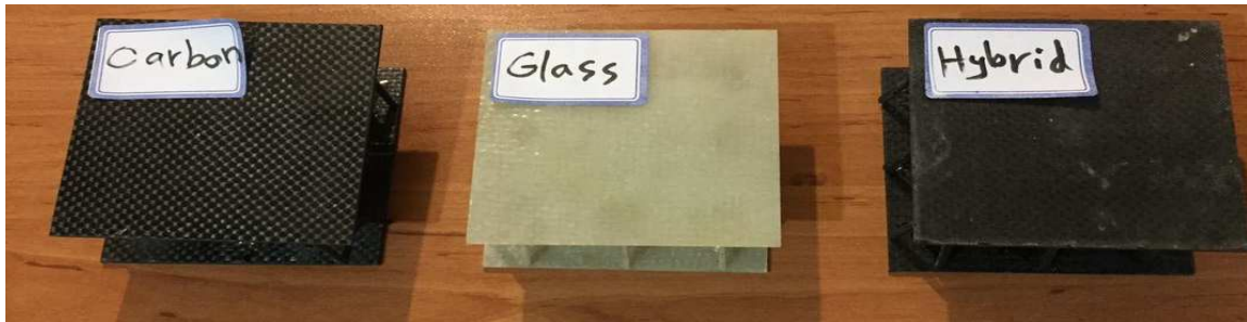
Fig.8. [C]_s , [G]_s , and [CGCG]_s composite sandwich panels
