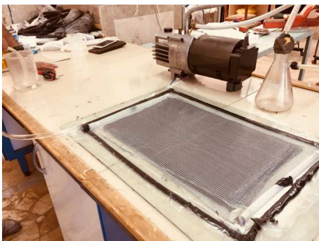
Fig.3. Vacuum bag pump
