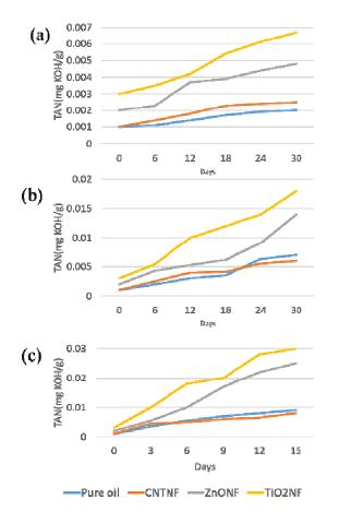
**Figure 1:** The results of TAN test for (a)110°C; (b)120°C; and (c) 130°C
