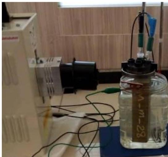
**Figure 3.** Placing the sample in sodium chloride solution for polarization and EIS tests.
