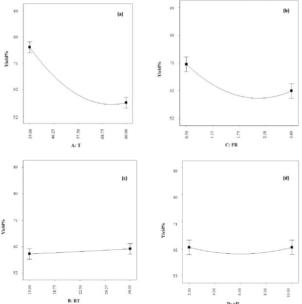
**Figure1.**Single-parameter effect on extraction efficiency.Chart of yieldin terms of: (a) Temperaturechanges under constant conditions:RT=22.5, FR=1.75, pH=6; (b) Flow intensity Ratio changes under constant conditions:RT=22.5, T=57.50, pH=6; (c) Residence Time changes under constant conditions:FR=1.75, T=57.50, pH=6; (d) pH changes under constant conditions:FR=1.75, PH=6; (d) pH changes under const
