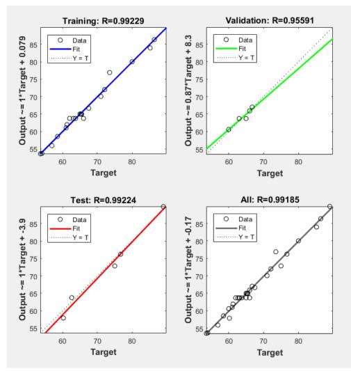
Figure 3.Performance R related to training, validation and testing, and all data in the proposed model by artificial neural network.
