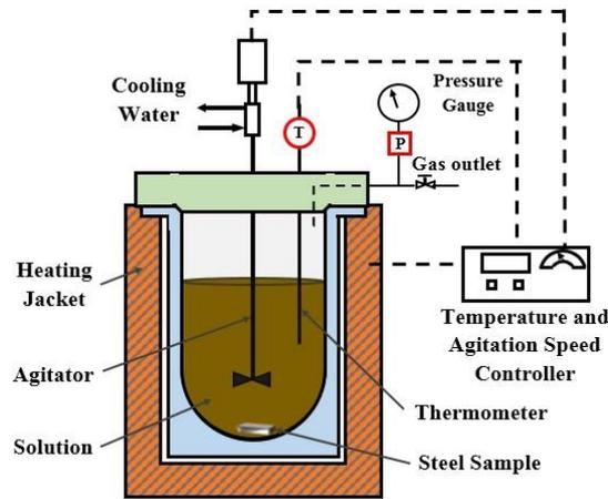
**Figure 2.** Schematic of autoclave used for corrosion test.
