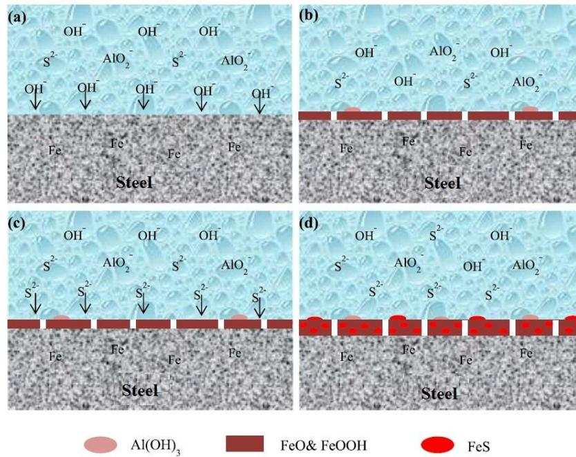
**Figure 6.** Corrosion mechanism of steel in sodium aluminate solution containing caustic soda and sulfide ions, **a**: Absorption of  $\text{OH}^-$  on steel surface, **b**: Passive film formation on steel surface, **c**: Adsorption of  $\text{S}^{2-}$  on the interface, **d**: Damage to the passive film and acceleration of corrosion.
