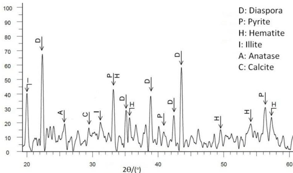
**Figure 3.** X-ray diffraction pattern of Jajarm Bauxite.
