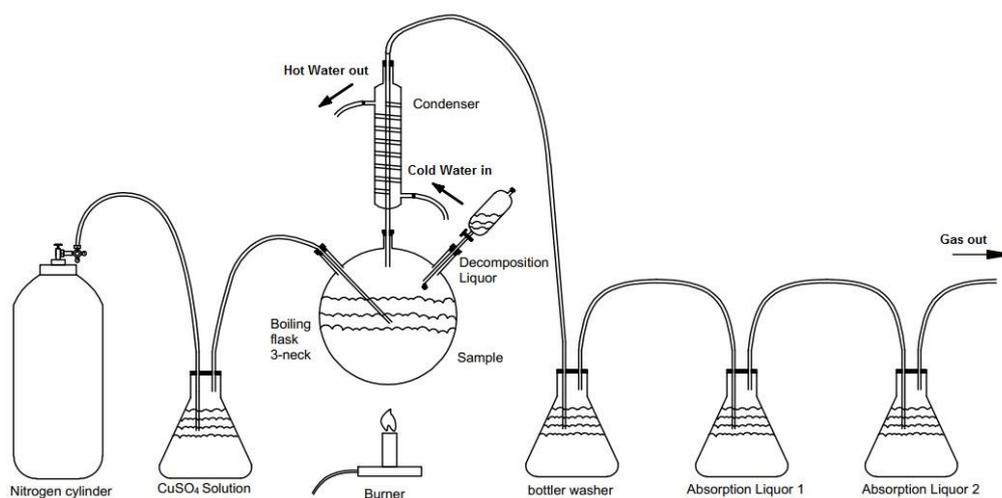
**Figure 1.** Schematic of the apparatus required for the separation of sulfide ions from the Bayer process aluminate solution.
