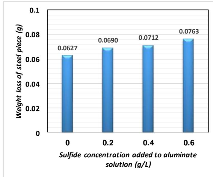
**Figure 4.** Weight loss of steel piece (corroded) in sodium aluminate solution with different concentrations of sulfide added.
