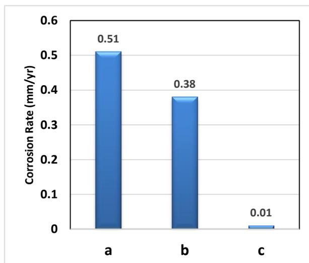
**Figure 7.** Comparison of carbon steel corrosion rate in: a - "Bayer process aluminate solution", b- "Bayer process aluminate solution + 2.5 g/L nitrate" and c- "0.2 g/L sulfide solution".
