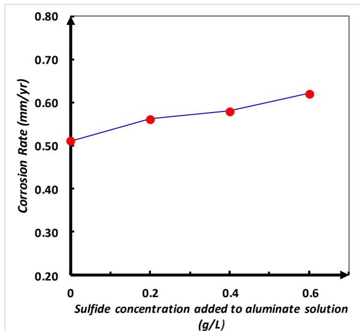
**Figure 5.** Corrosion rate of carbon steel piece in aluminate solution with different concentrations of added sulfide.
